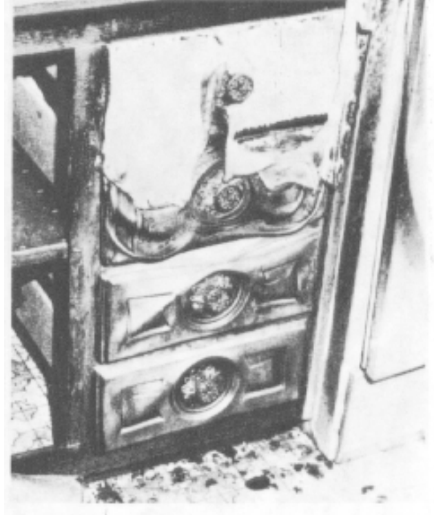
The plastic drawer fronts lack the fire resistance of the wood they simulate, and some synthetic garments burn furiously.
